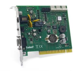
The module supports several transmission formats with automatic recognition and autonegotiation of the communication protocol. The amount of data received by the card is unlimited and their correctness is tested as they come. The card has a FIFO buffer for 250 last received events.
